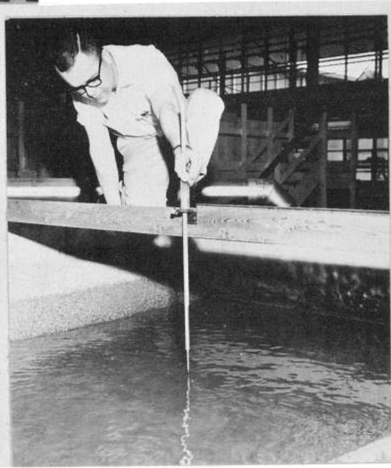
C. Point gage for determining water surface elevation in canal.
