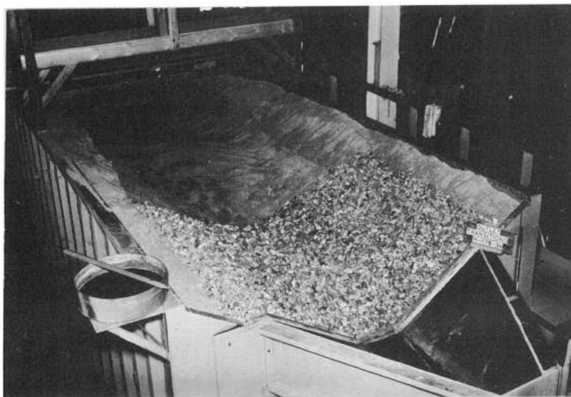
FIGURE 19.—Flow and scour in canal protected by 4-inch layer of 1\frac{1}{2} -inch gravel, 1 to 8 slope, 6-inch rise transition with warped walls and horizontal pipeline, outlet flows.
