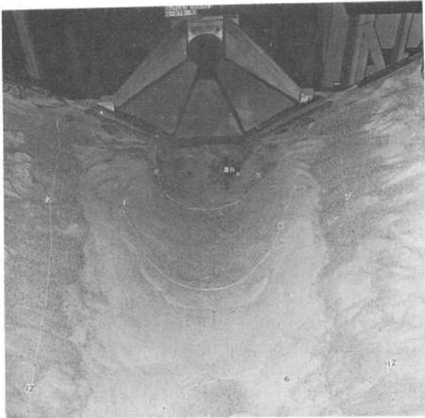
B. Scour after 30 minutes operation each at flow velocities in pipeline of 2, 2.5, and 3 f.p.s., depth=0.8 D.
