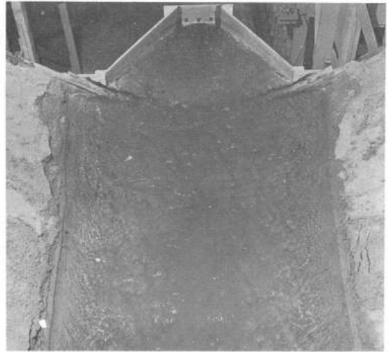
A. Mildly turbulent water surface. Q=2.4 c.f.s., V_p=3.0 f.p.s., depth=0.8 D.
