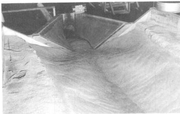
B. Scour after 1 hour operation. Q=2.4 c.f.s., V_p=3.0 f.p.s., depth =1.3 D . Sand was deposited in the transition.
