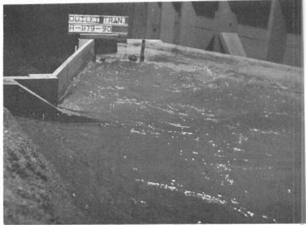
A. Turbulent water surface. Q=2.4 c.f.s., V_p=3.0 f.p.s., depth=0.8 D.
