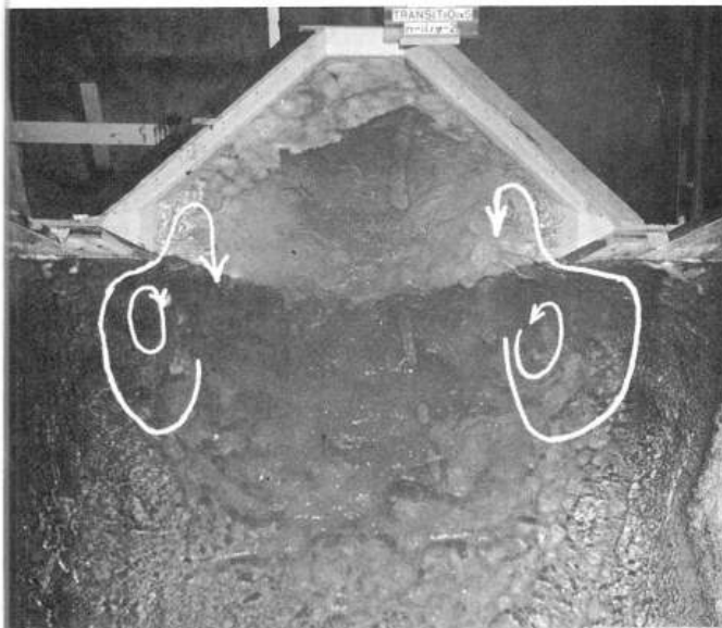
A. Flow is confined mainly to passage center. Eddies occur at sides. Q=3.0 c.f.s., V_p=3.8 f.p.s., canal depth =1.5 D .
