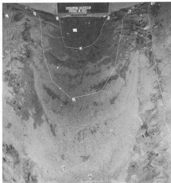
C. Scour after 1 hour operation. V_p=6.0 f.p.s., canal depth=1.25 D.
