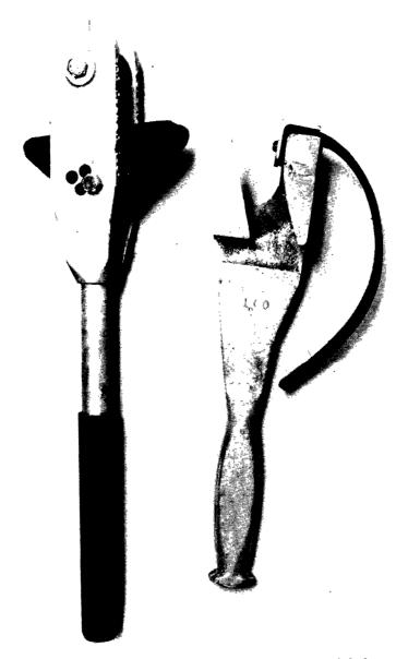
FIGURE 69.—Cable-car puller for follower-brake cable cars, left; for standard cars, right.
