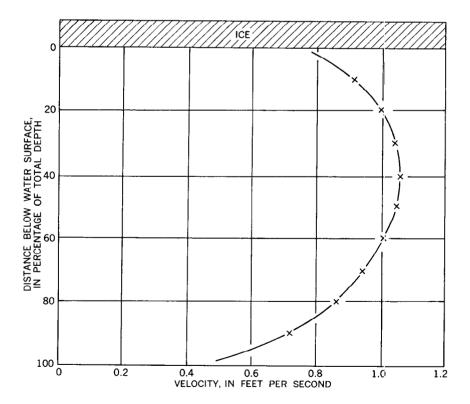
FIGURE 95.—Typical vertical-velocity curve under ice cover.
