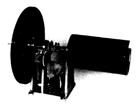
FIGURE 33.—Resistance system transmitter unit.
