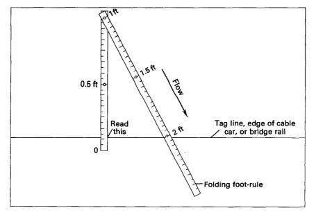
FIGURE 91.—Measurement of horizontal angle with folding foot-rule.
