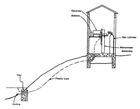
FIGURE 31.—Typical bubble-gage installation.
