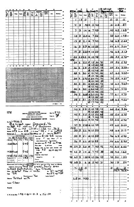
FIGURE 42.—Computation notes of a current-meter measurement by the midsection method.
