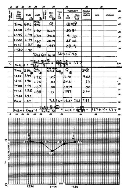
FIGURE 101.—Computation of discharge-weighted mean gage height.
