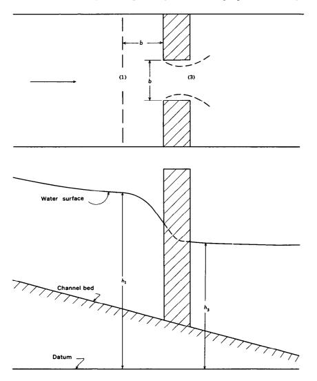
FIGURE 135.—Definition sketch of an open-channel contraction.
