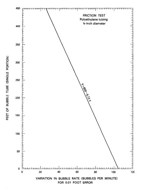
$\label{Figure 36.} \textbf{Figure 36.--Diagram for determining allowable length of bubble tubing for maximum friction error of 0.01 ft.}$
