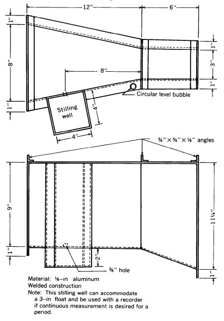
FIGURE 130.—Working drawing of modified 3-in Parshall flume.
