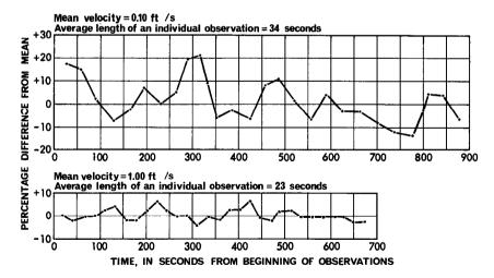
FIGURE 43.—Comparison of pulsations for two different mean velocities measured in a laboratory flume, 12 ft wide.
