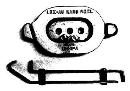
FIGURE 63.—Handline reels: Lee-Au (top) and Morgan (bottom).
