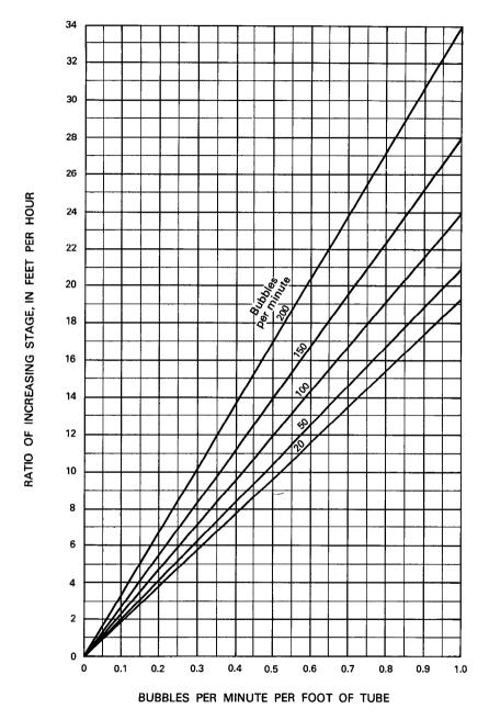
FIGURE 37.—Diagram for determining required bubble rate.
