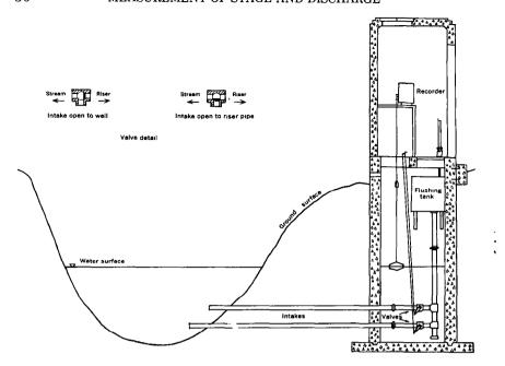
FIGURE 29.—Flushing system for intakes.
