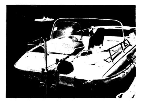
FIGURE 110.—Boat with mounted vane assembly.
