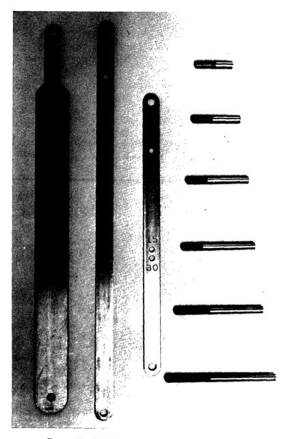
FIGURE 57.—Sounding-weight hangers and hanger pins.
