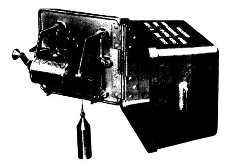
FIGURE 10.—Type A wire-weight gage.
