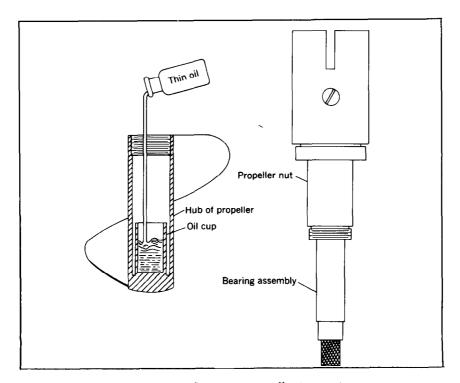
FIGURE 106.—Component propeller-type meter.
