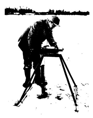
FIGURE 84.—Collapsible reel support and ice-weight assembly.
