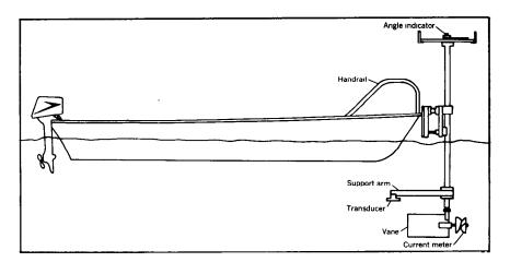
FIGURE 105.—Sketch of boat showing equipment.
