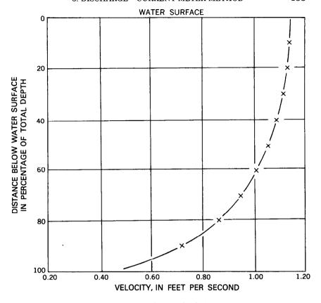
FIGURE 88.—Typical vertical-velocity curve.
