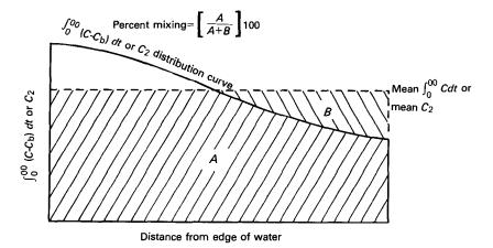
FIGURE 119.—Concentration-distribution curve illustrating the graphical method of determining the percentage of mixing.
