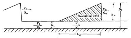
FIGURE 132.—Schematic sketch of longitudinal water-surface profile during pulsating flow.
