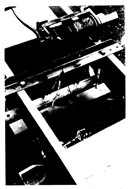
$\begin{tabular}{ll} F_{\sc IGURE} \sc 72. \label{table} - Portable \ reel \ seat \ on \ sit down-type \ cable \ car. \ (Note \ tags \ on \ sounding \ cable.) \end{tabular}$
