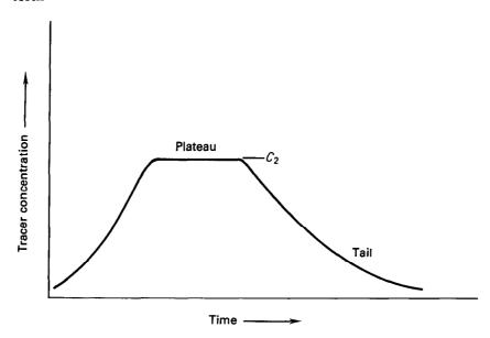
FIGURE 116.—Concentration-time curve at downstream sampling site for constantrate injection.
