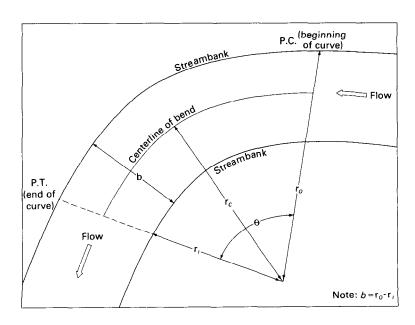
FIGURE 138.—Idealized sketch of a bend (plan view).
