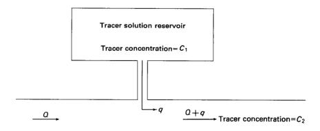
FIGURE 115.—Constant-rate-injection system.
