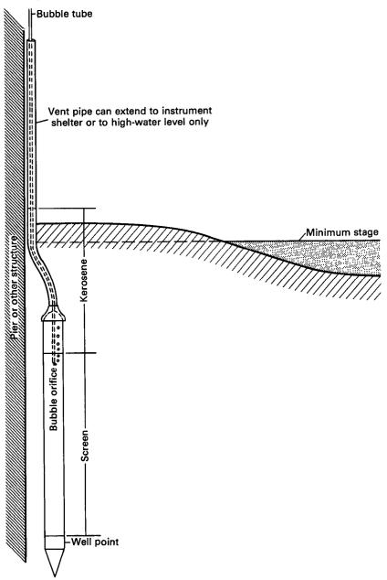
FIGURE 15.—Installation of bubble orifice in unstable streambed.
