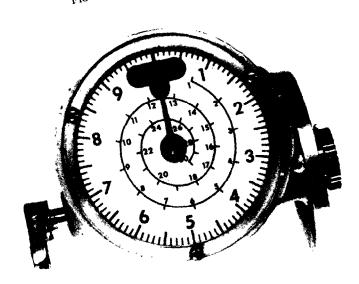
FIGURE 60.—Computing depth indicator.
