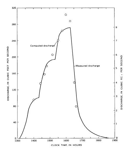
FIGURE 133.—Discharge hydrograph at Santa Anita Wash above Sierra Madre Wash, Calif., April 16, 1965, and plot of discharges computed from observations of flow.
