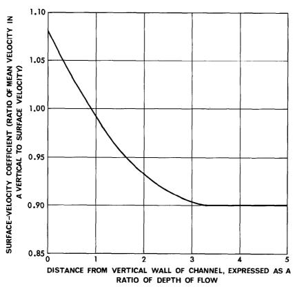
FIGURE 89.—Relation of surface-velocity coefficient to distance from vertical wall of a smooth rectangular channel.
