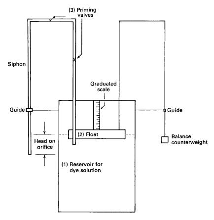
FIGURE 122.—Floating siphon (constant-head device).
