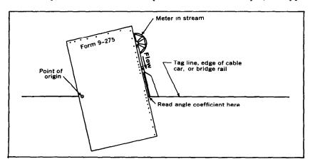
FIGURE 90.—Measurement of horizontal angle with measurement-note sheet.
