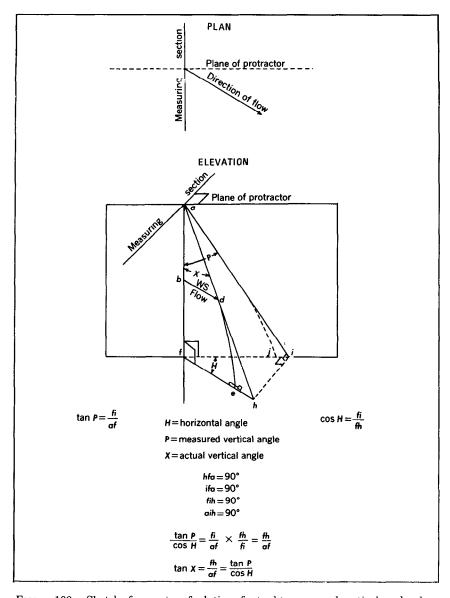
FIGURE 100.—Sketch of geometry of relation of actual to measured vertical angle when flow direction is not normal to measurement section.
