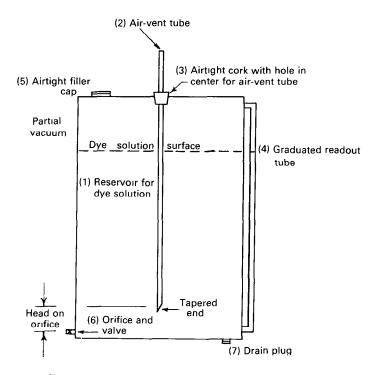
FIGURE 121.—Mariotte vessel (constant-head device).
