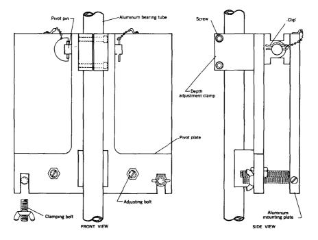
FIGURE 111.—Detailed view of vane-mounting assembly.
