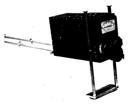
FIGURE 50.—Optical current meter.
