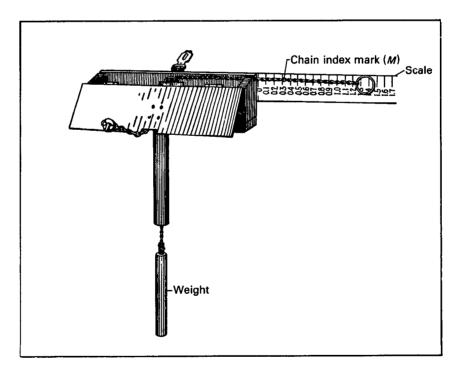
FIGURE 13.—Chain gage (cantilevered mount not shown).
