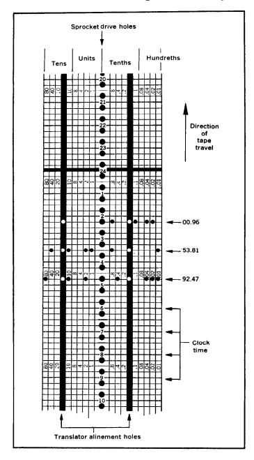
FIGURE 17.—Sample digital-recorder tape.
