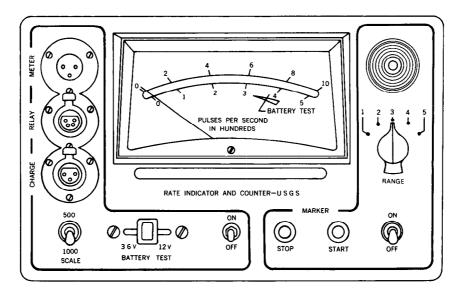
FIGURE 107.—Control panel of rate indicator and counter.
