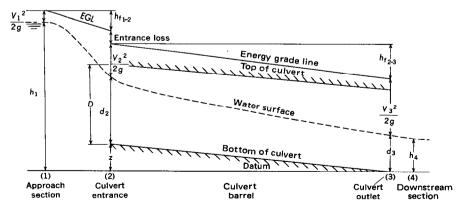
FIGURE 136.—Graphical presentation of the Bernoulli equation in culvert flow.
