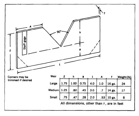
FIGURE 129.—Portable weir-plate sizes.
