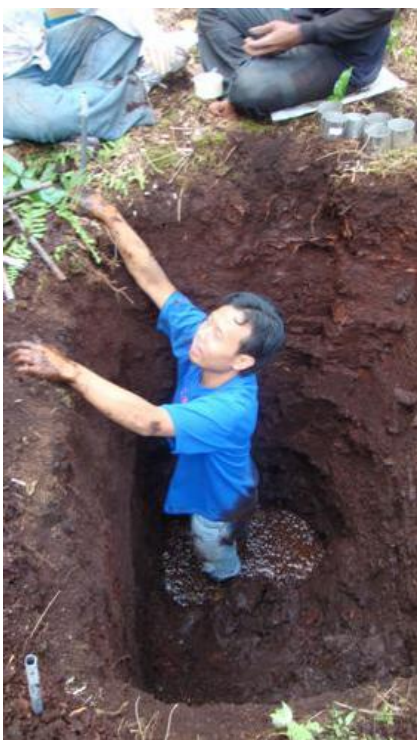
Peat sampling: ring samples from pits
