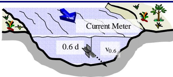
Velocity Measurement by Current Meter
