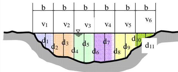
Measurement of Sectional Area & Velocity
