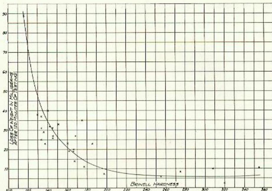
Fig. 13—Effect of hardness of various welded materials on resistance to pitting.
