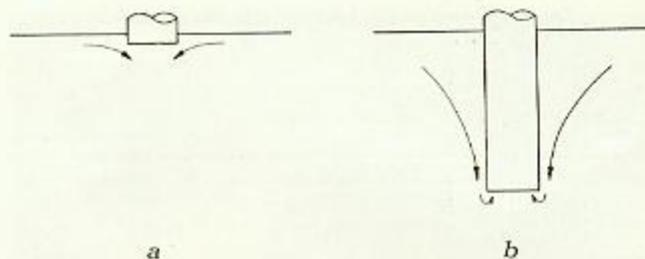
Fig. 17—Flow of liquid below test specimen according to Rightmire.
