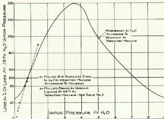
Fig. 11—Relation between vapor pressure and rate of pitting as measured by loss of metal in test specimen.
