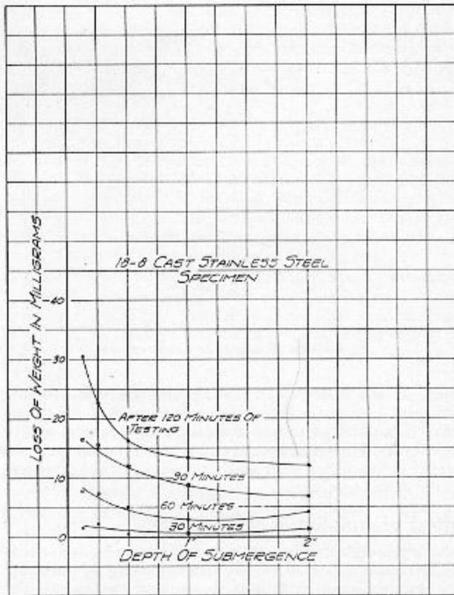
Fig. 7—Cavitation tests to determine effect of submergence on stainless steel specimens.
