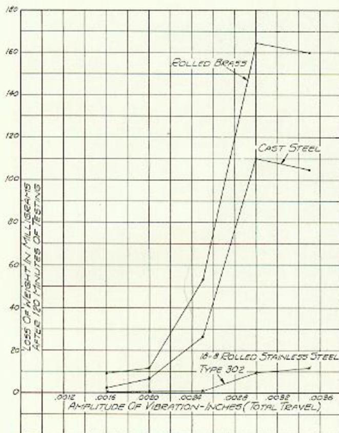
Fig. 5—Effect of amplitude on vibration.
