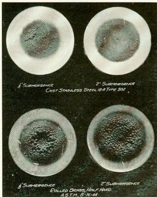
Fig. 8—Photograph of brass and stainless steel at  $\frac{1}{8}$  in. and 2 in. submergence.
