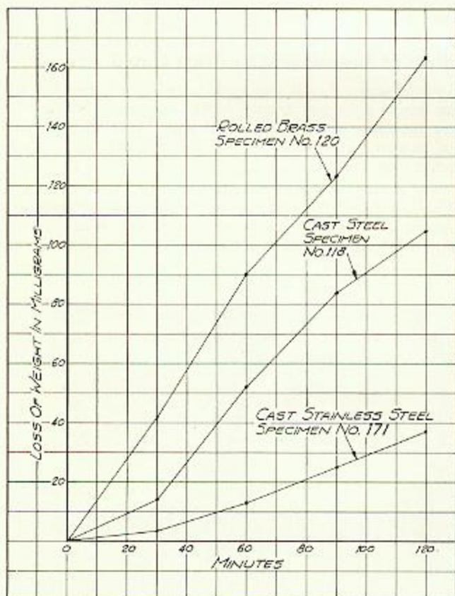
Fig. 4—Loss of weight of test specimens.
