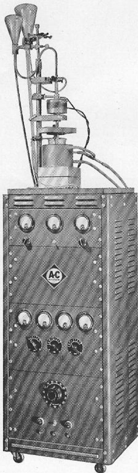
Fig. 2—Photograph of accelerated cavitation test machine.
