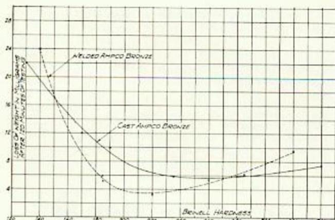
Fig. 15—Effect of hardness of Ampco bronzes on resistance to pitting.
