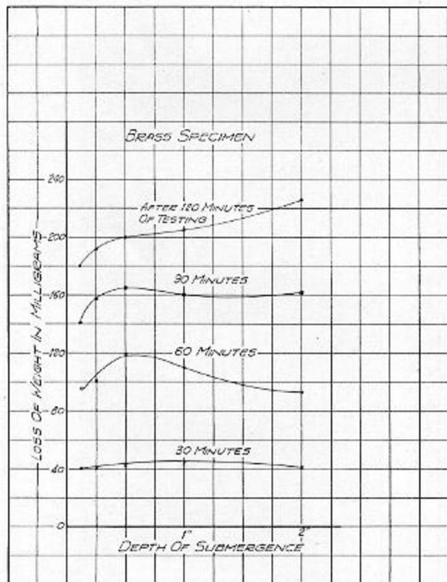
Fig. 6—Cavitation tests to determine effect of submergence on brass specimen.
