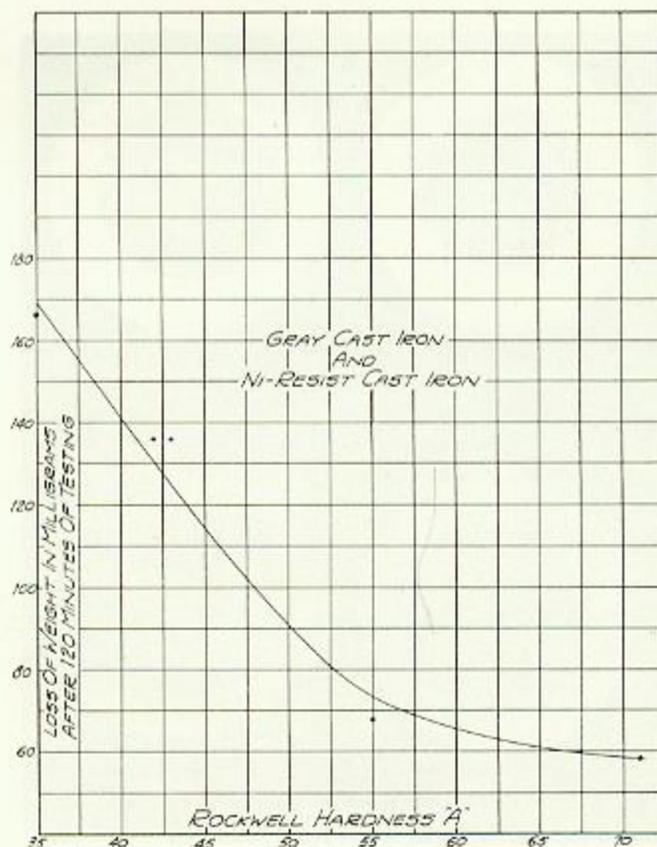
Fig. 10—Effect of hardness of cast iron on resistance to pitting.
