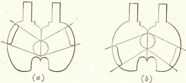
FIG. 84.—Radii for different bucket positions.
