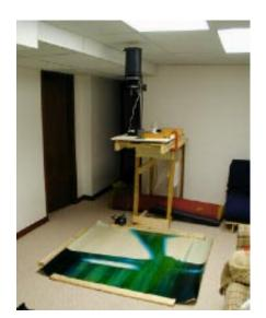
The enlarger's position is also very important: the shelf and negative holder levels were checked against the floor level many times during the printing session. They have to be the same so the picture appears as a rectangle, not some other geometrical form!
