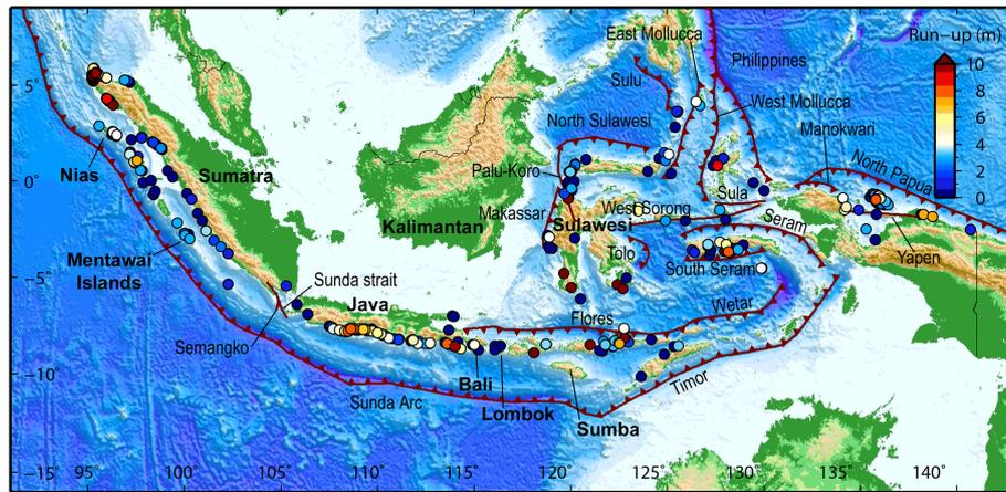
**Figure 1.** Map showing the local sources (red lines, thin black text) used in the PTHA and historical tsunami run-up observations (coloured circles) from Latief et al. (2000) and the NOAA NGDC database. Geographic locations referred to in the text are in bold black font.
