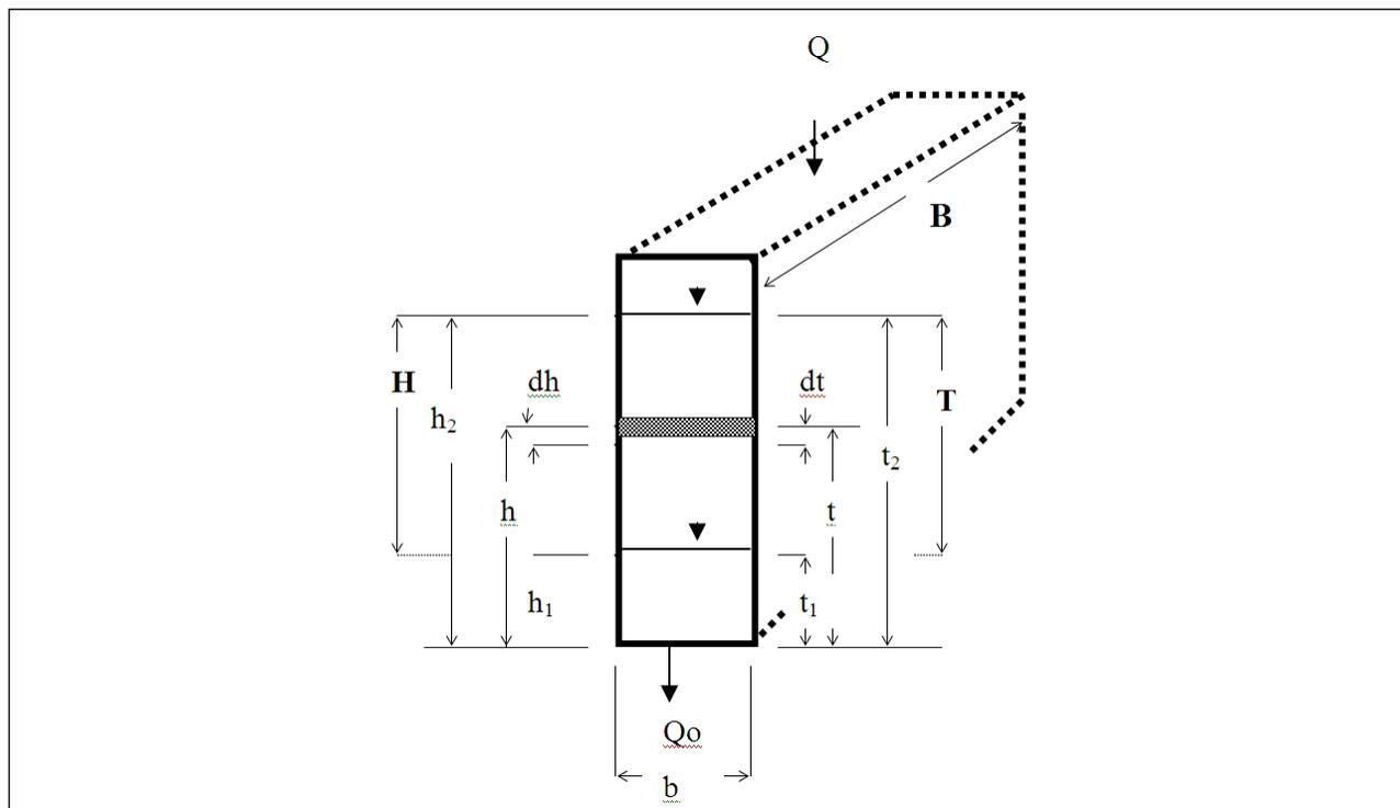
Figure 2. Sketch of water balance for the trench.
