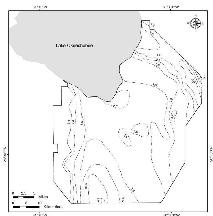
**Fig. 4.** Contour map of bedrock elevation (ft, NGVD29) for the EAA. From Parker et al. (1955).
