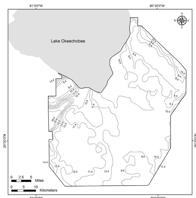
**Fig. 6.** Contour map of current peat surface elevation (ft, NGVD29) for the EAA, ca. 2005.
