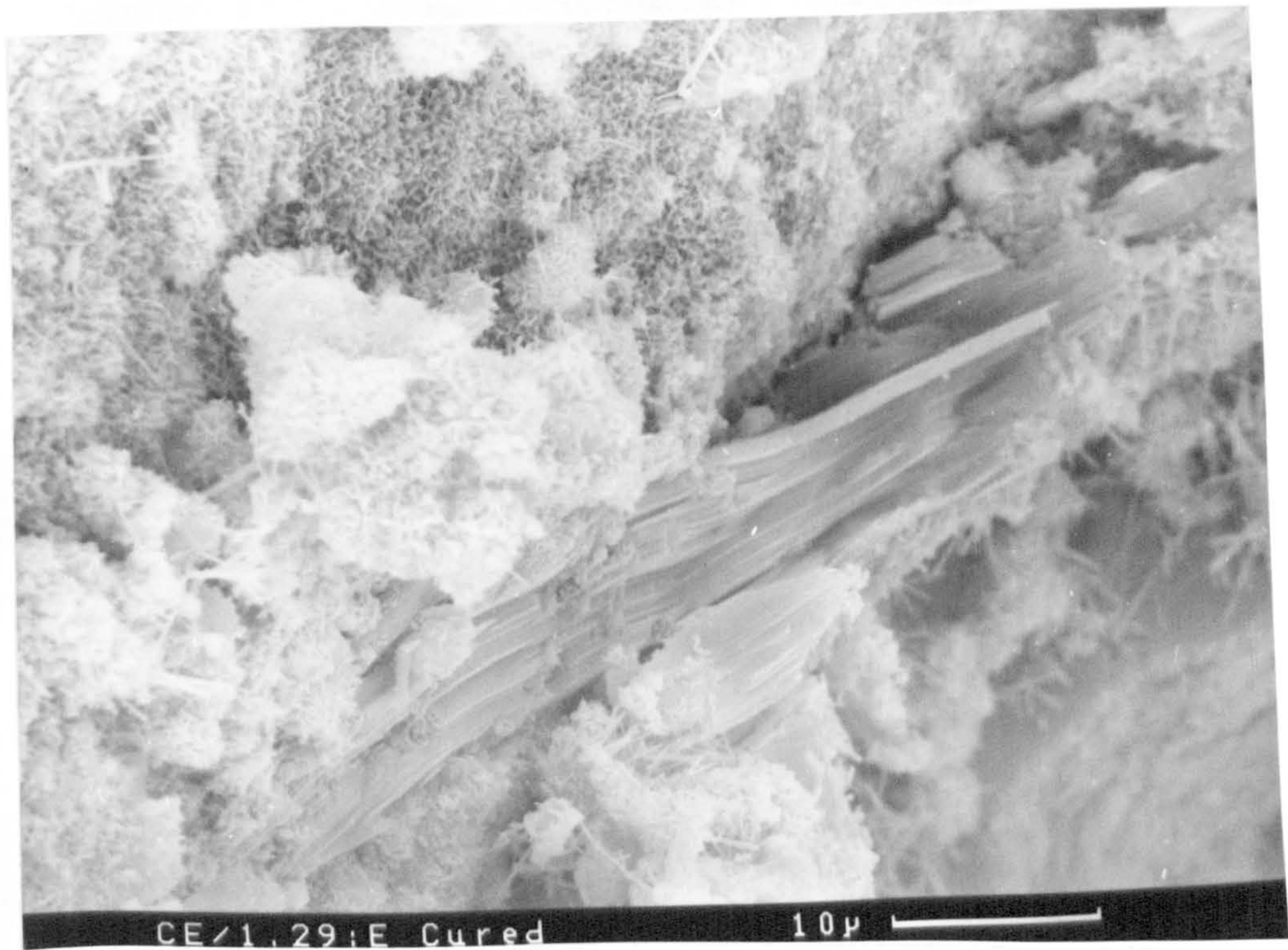
Plate 9.11 SEM micrograph illustrating a typical fracture surface of mortar mix number 21 (Magnification \times 1900 ). The massive calcium hydroxide deposits grown through regions of C-S-H gel is clearly seen.
