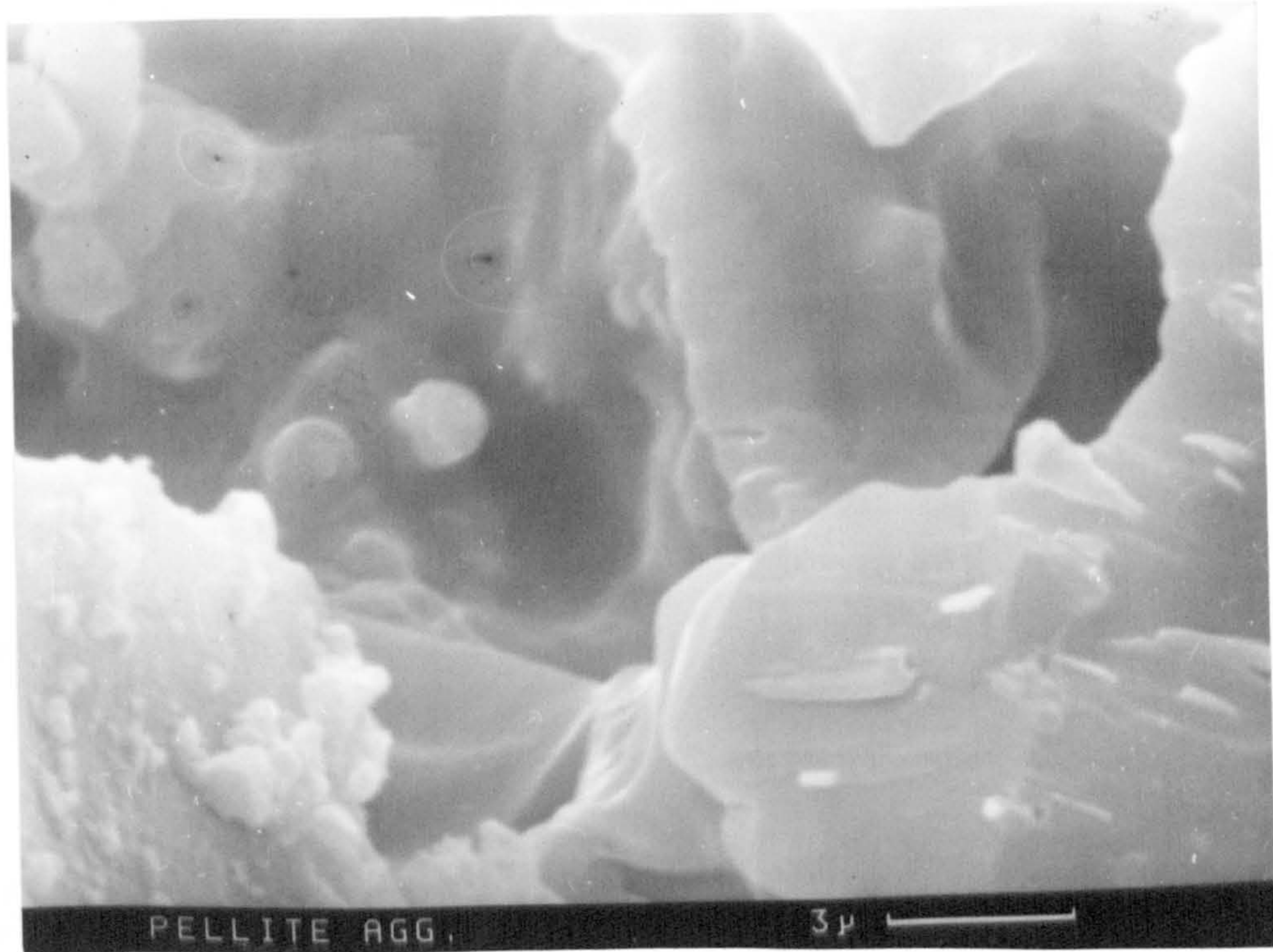
Plate 9.9 General view of the fracture surface of Pellite aggregate showing a close-up view of an area marked in Plate 9.8 magnification \times 5750
