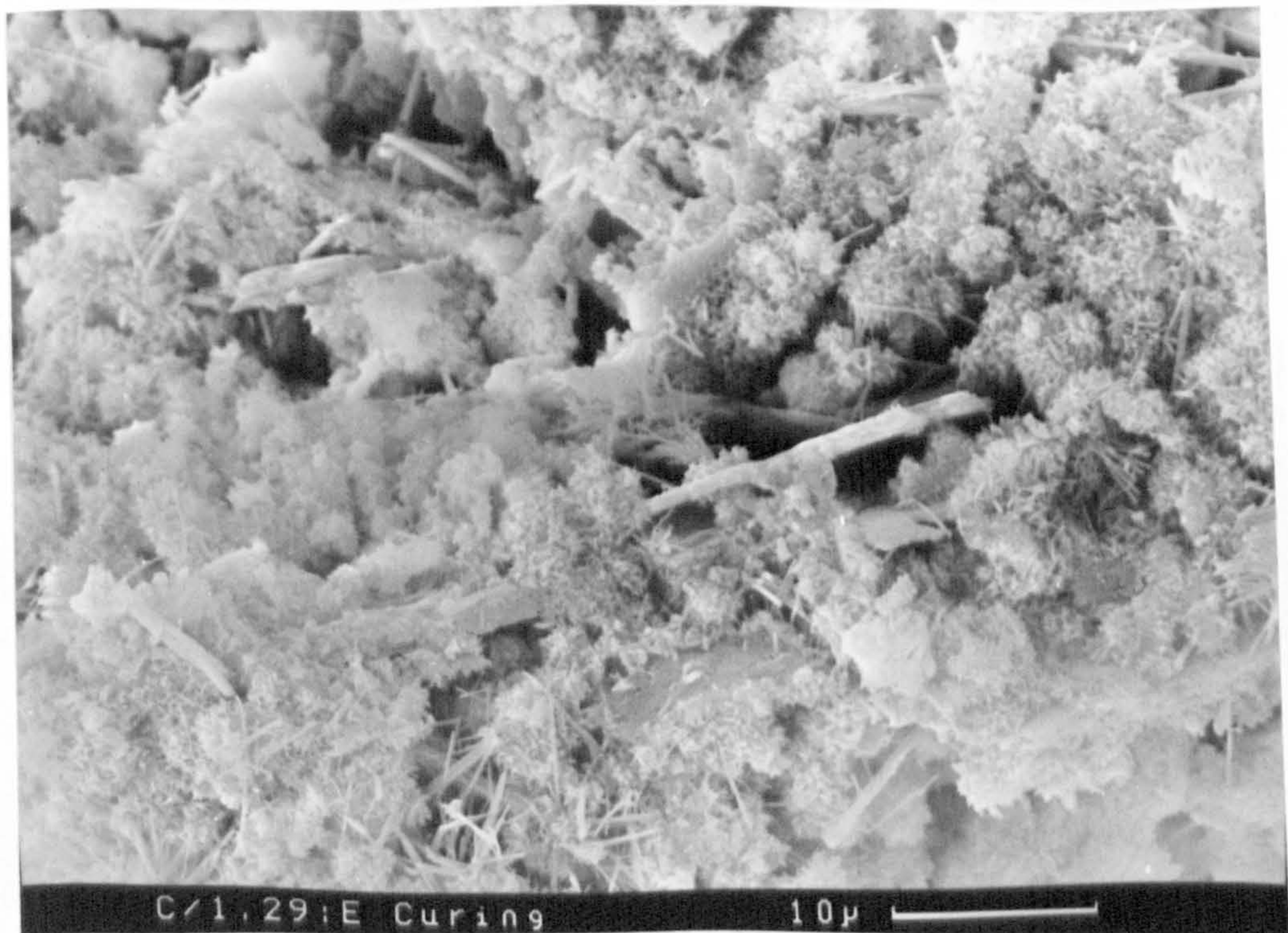
Plate 9.10 SEM micrograph illustrating a typical fracture surface of mortar mix number 20 (Magnification \times 1920 ). The C-S-H gel (honeycomb morphology) are visible in this micrograph.
