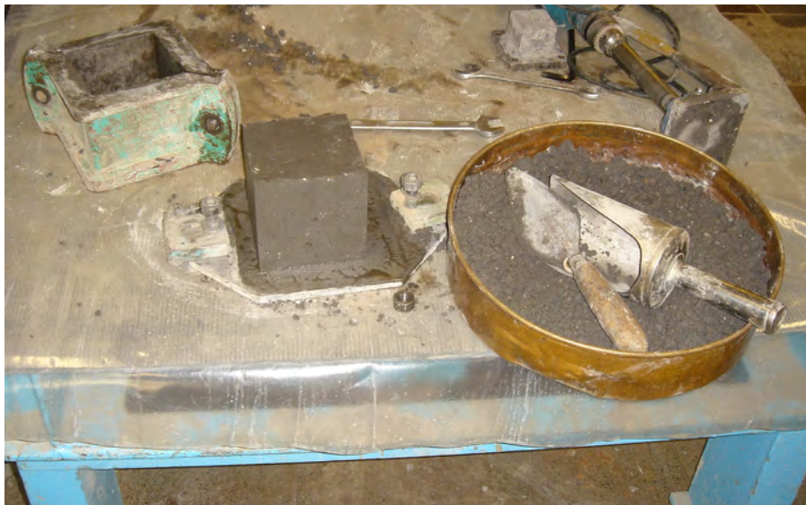
Figure 6-13 Fresh light weight concrete demoulded straight after concrete casting
