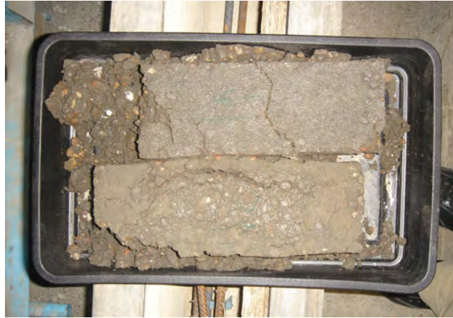
Figure 4- 31 Sample BOS 30%-ROSA 60%-RG 10% burst after 10 freeze-thaw cycles
