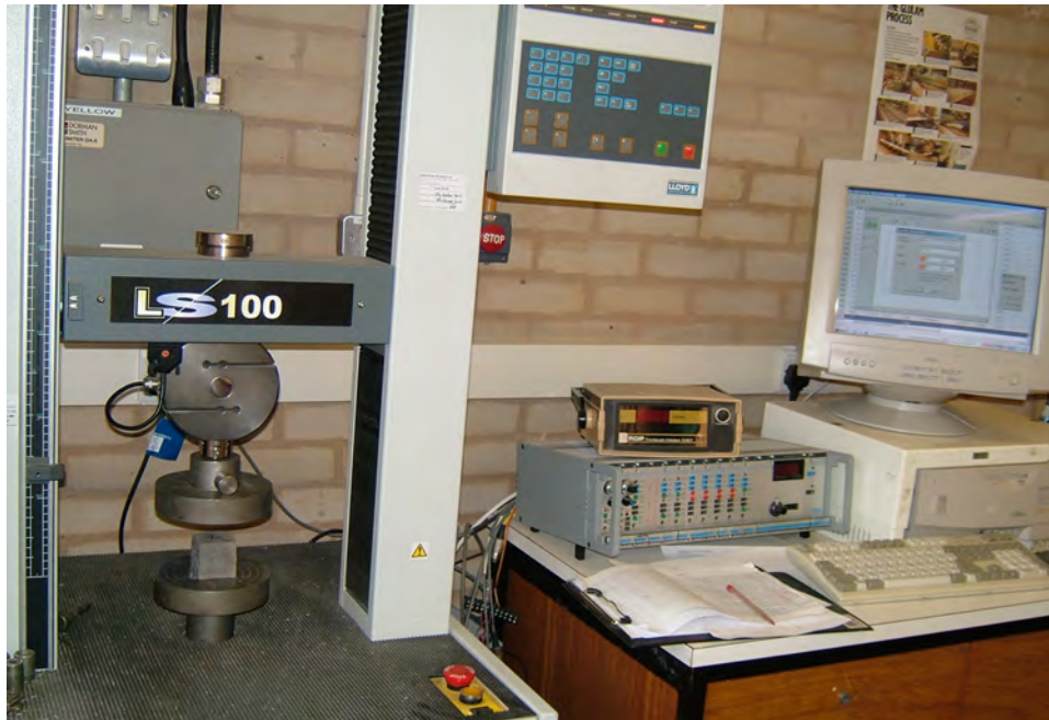
Figure 3- 14 Lloyd computerised compressive strength testing machine
