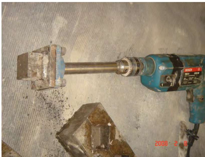
Figure 6- 5 Sample compaction using hammer drill for 50 mm cube
