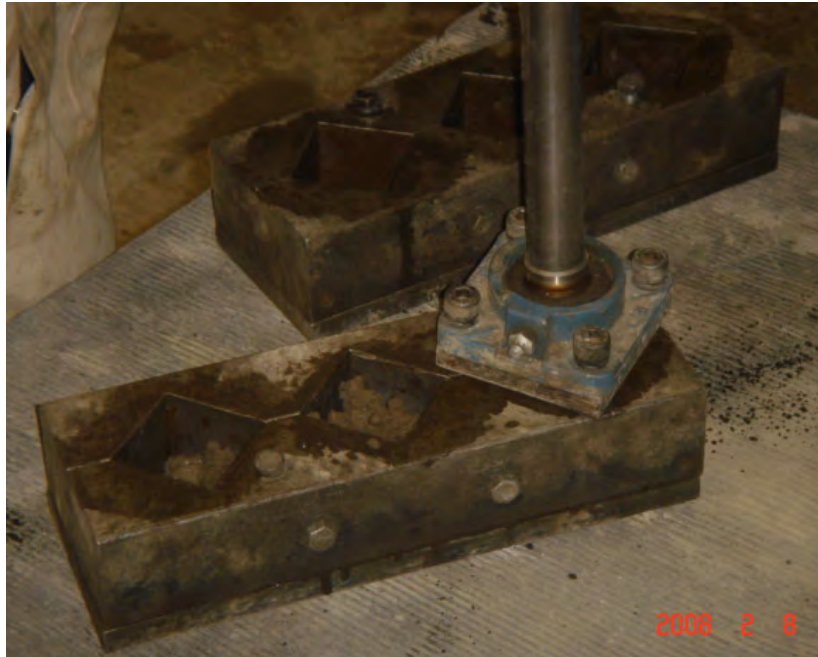
Figure 6- 5 Sample compaction using hammer drill for 50 mm cube
