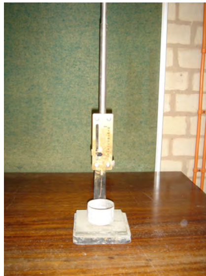
Figure 3- 10 Vicat Apparatus for determining the setting time of mortar
