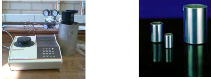
Figure 3- 3 Micromeritics AccuPyc 1330 Helium Pycnometer and Sample Cells
