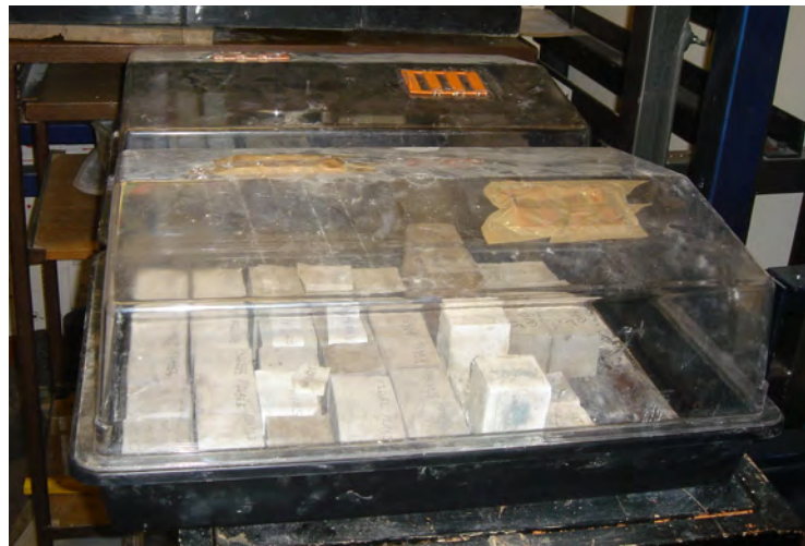
Figure 3-13 Sample curing container
