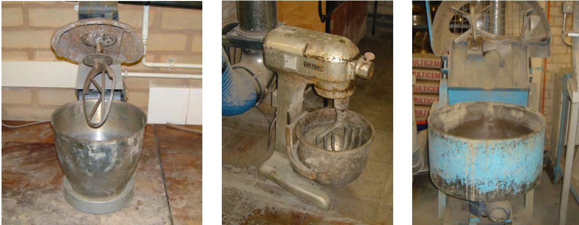
Figure 3- 5 From left: 2-litre mixer, 10-litre mixer, horizontal mixer
