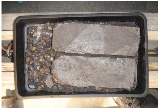
Figure 4- 32 Sample BOS 30%-ROSA 60%-PG10% burst after 10 freeze-thaw cycles
