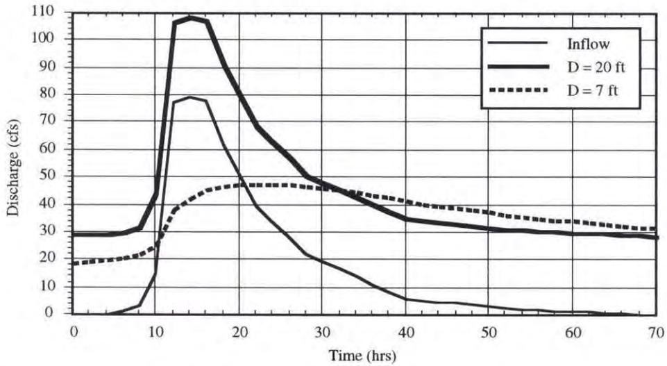
Figure 7. Discharge Hydrographs at Big Spring for Megapore Diameters, D, 7 ft and 20 ft.
