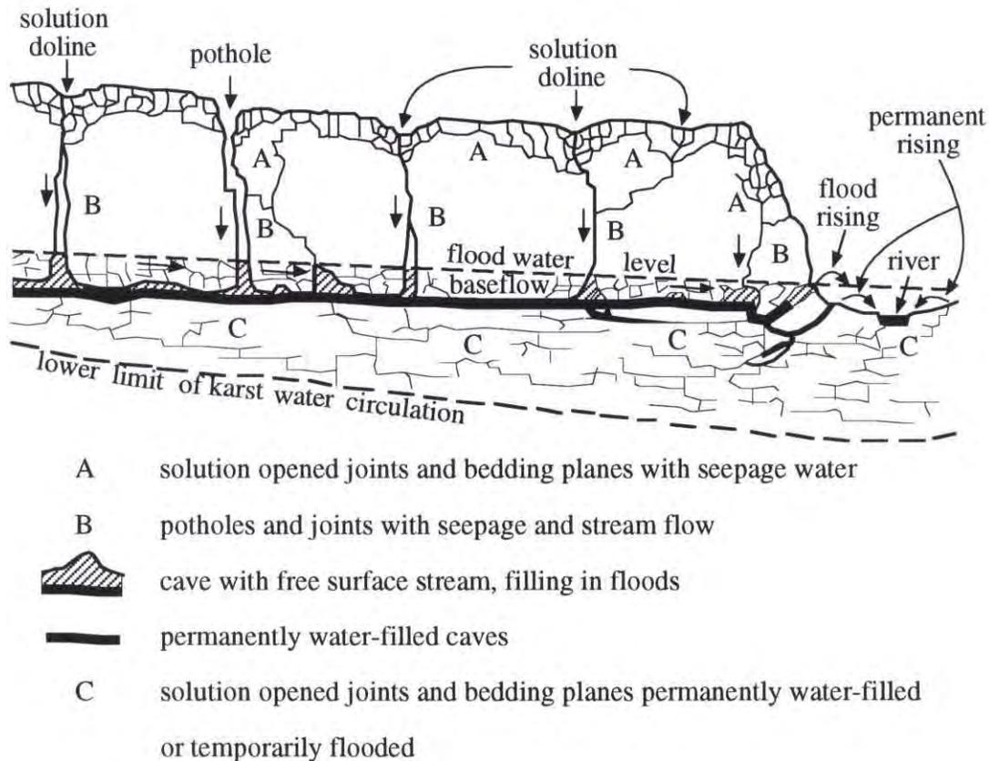
Figure 1. A Karst Hydrologic System Based on the Concept of Independent Conduits, after Cavaille (1962)
