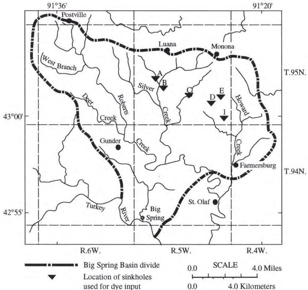
Figure 6. Location of Sinkholes Used for Dye Trace Experiments, after Hallberg et al. (1983)
