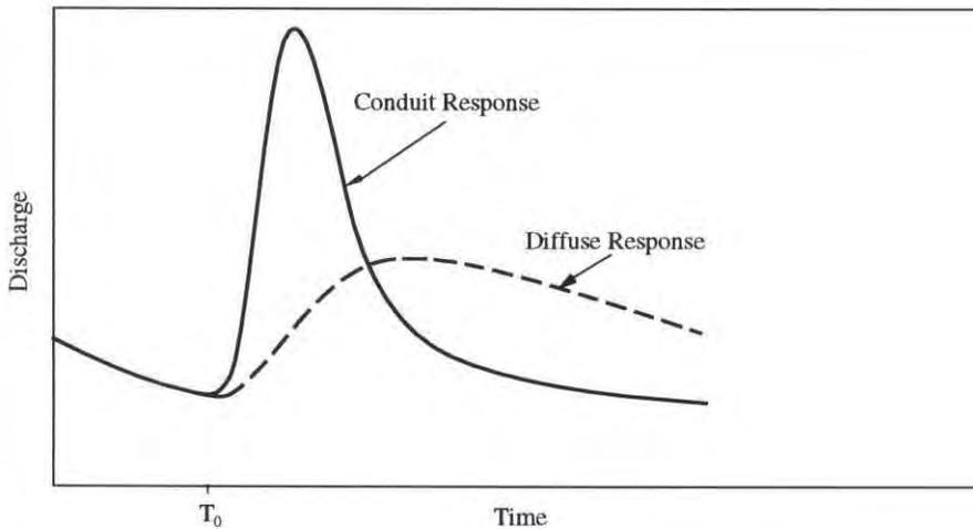
Figure 8. Schematic Hydrographs Showing the Difference between Conduit-Flow and Diffuse-Flow Discharge in a Carbonate Aquifer (e.g., at a spring) over Time, in Response to a Recharge Event at Time,  $T_0$ , after Hallberg et al. (1983).
